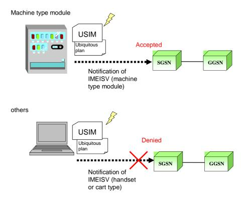
Figure A-3: Access Control with billing plan
