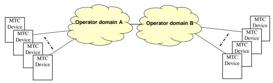
Figure 5-3: MTC Devices communicating directly with each other without intermediate MTC server.
