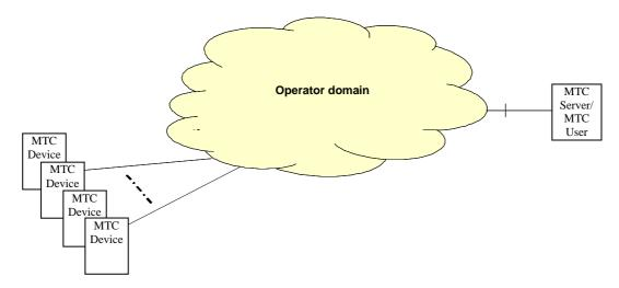
Figure 5-2: Communication scenario with MTC devices communicating with MTC server. MTC server is located outside the operator domain.
