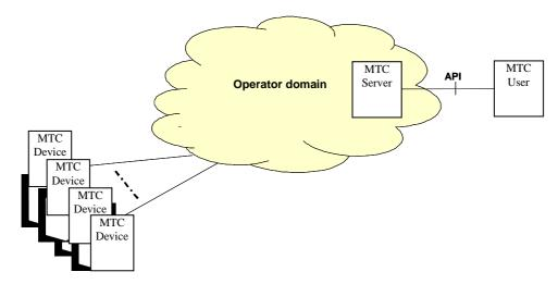
Figure 5-1: Communication scenario with MTC devices communicating with MTC server is located in the operator domain.
