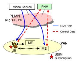
Figure 7: Single network connection through PNE holding the (U)SIM of PAN
