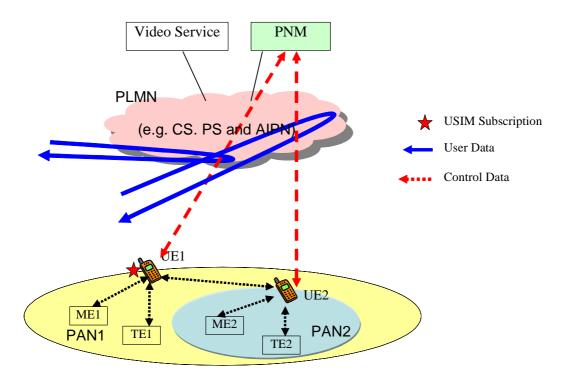
Figure 13: Combination of two PANs (case 1)
