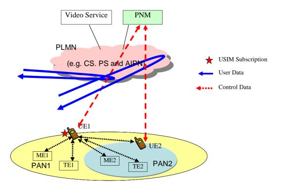
Figure 14: Combination of two PANs (case 2)
