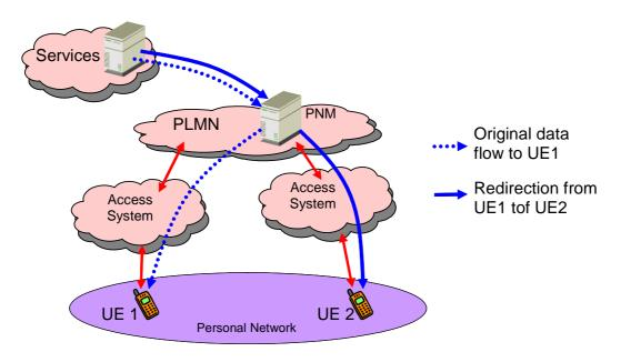
Figure 11: Activation of UE 2 for directing service termination to UE 2
