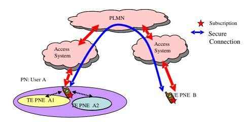
Figure 6: Use case for UE-PN connection
