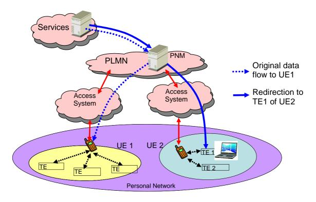
Figure 12: Activating a particular device of a UE or PAN for service termination
