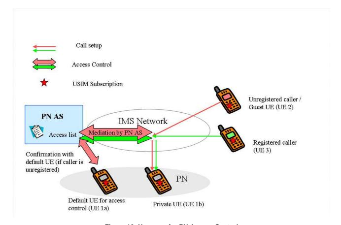
Figure 16: Use case for PN Access Control
