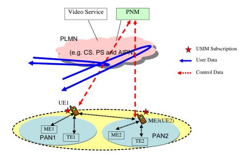
Figure 15: Separation of PAN
