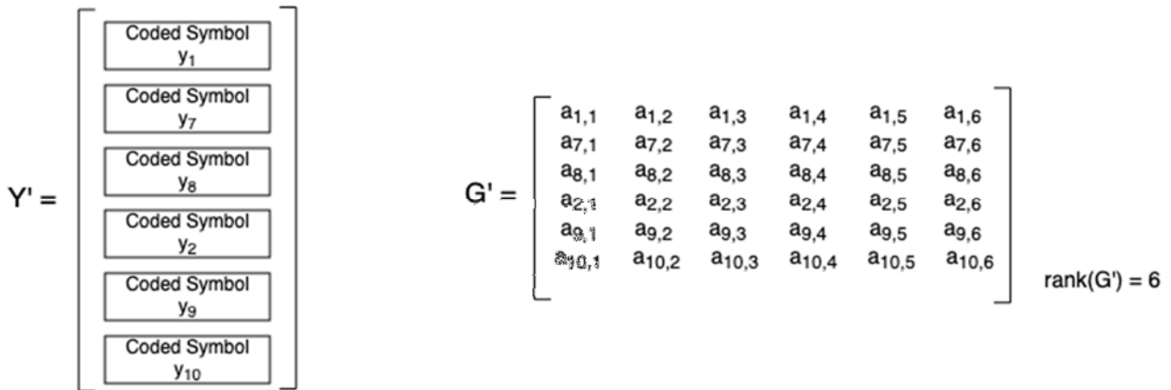
Figure A.4: xCD-1 coded symbol vector and decoded coefficient matrix
