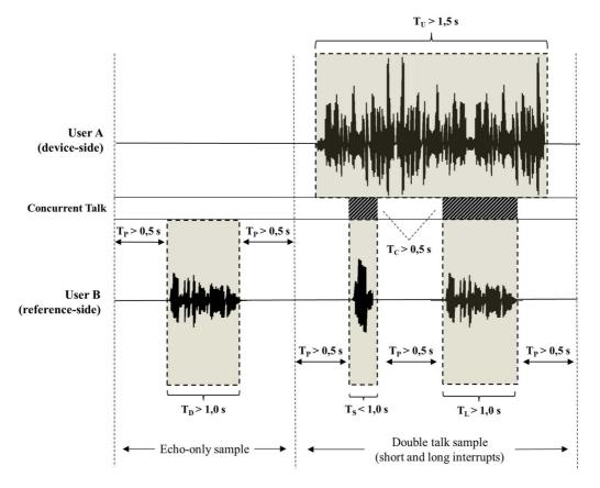
Figure 4: Example of source signal for generation of TPLT samples
