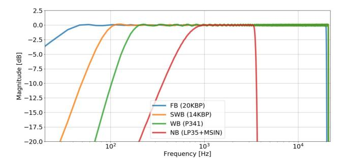
Figure B.1: Transfer functions of Recommendation ITU-T G.191 [26] filters
