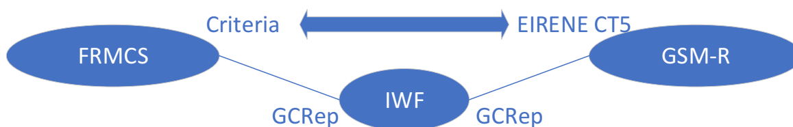
Figure 6.3.3.5.0-1: Coupled FRMCS/GSM-R Group Call
