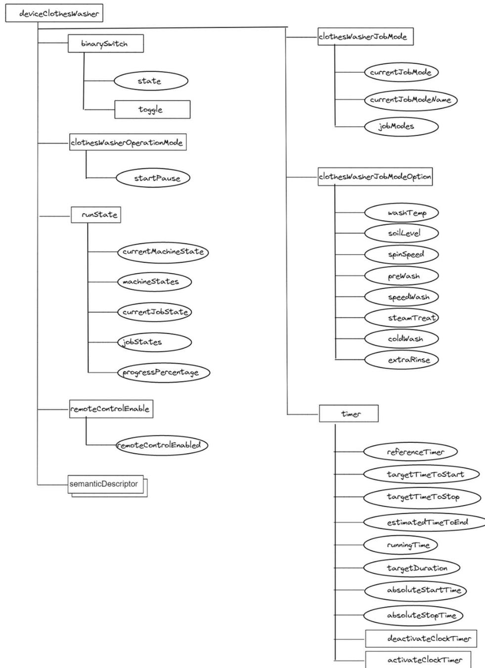
**Figure 9: SDT washing machine model**
