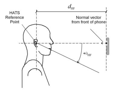
Figure 5.2.1-1: Configuration of handheld hands-free UE relative to the HATS
