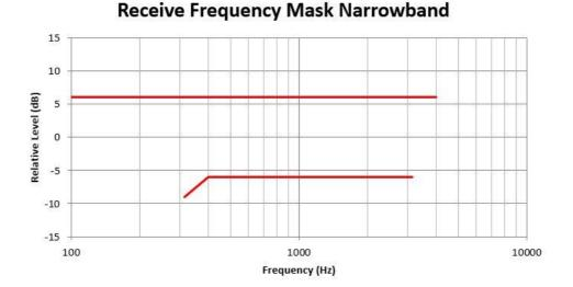
Figure 6.1.2.4-1: Desktop terminal receive sensitivity/frequency response
