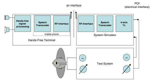
NOTE: The "whole" terminal includes all the components from "RF interface" to the transducers and may include an additional (radio) link. The air interface considered in figure 5.1-1 is not the additional radio link.
