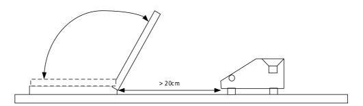
Figure 5.2.5-1: Positioning of DUT
