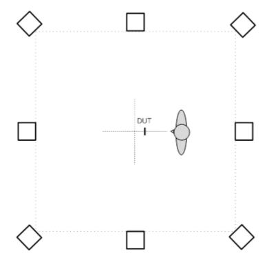
Figure 5.5.3-1: Loudspeaker arrangement for background noise simulation
