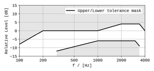
Figure 6.1.1-1: Hands-free send sensitivity/frequency response
