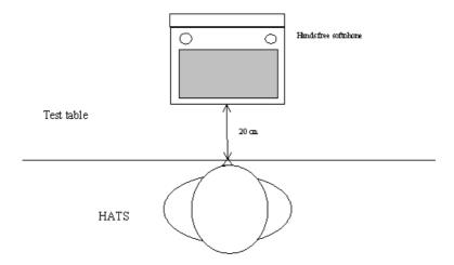
Figure 5.2.4.1-2: Configuration of softphone relative to the HATS-top sight
