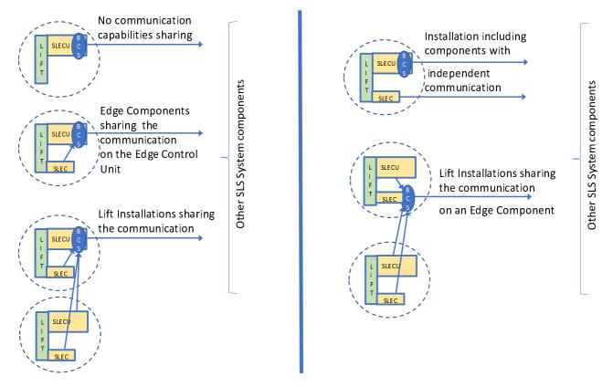
Figure 5.2-1: Smart Lift deployment cases
