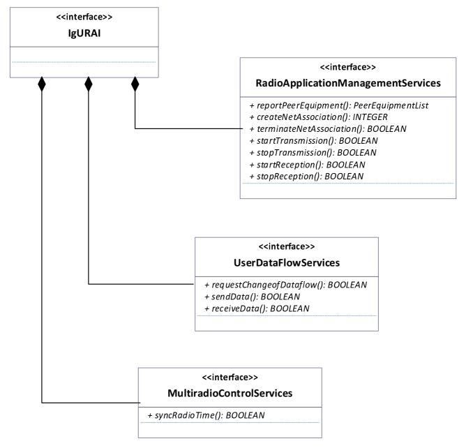
Figure 8.1: UML diagram for gURAI
