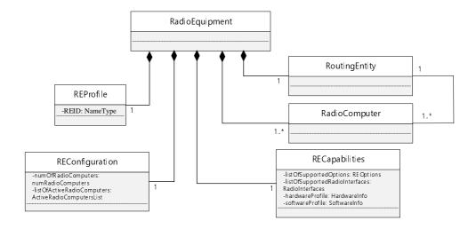
NOTE: The Routing Entity this figure is responsible for transferring command/information to/from corresponding radio computers. An (external) network controller may be able to update the routing path to radio computers by accessing Routing Entity through a propoer interface. An (external) network controller and an interface are vendor-specific and out of scope of the present document.
