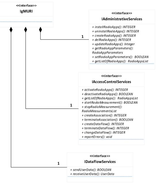
Figure 8.2: UML diagram for gMURI
