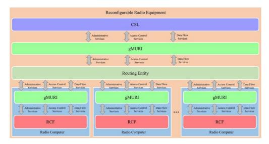
Figure 5.1: Interconnection between CSL and RCF using gMURI for Reconfigurable RE
