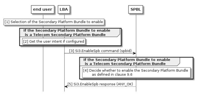
Figure 12.10: Enable Secondary Platform Bundle procedure
