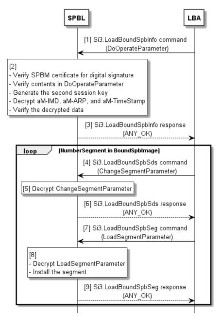
Figure 12.9: Installation procedure
