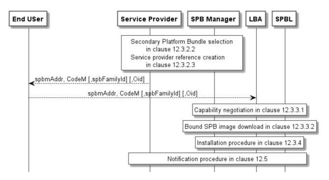
Figure 12.2: Secondary Platform Bundle provisioning procedure - case 1
