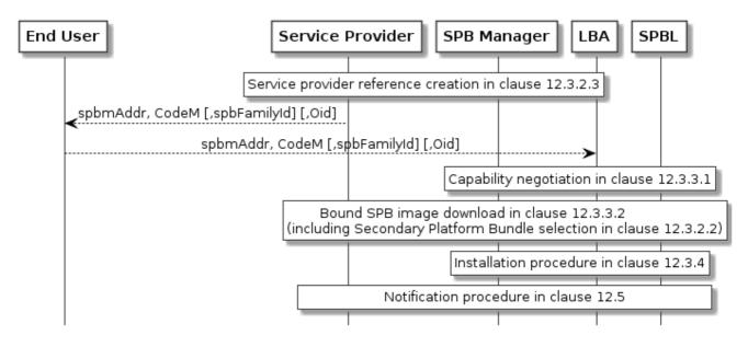
Figure 12.3: Secondary Platform Bundle provisioning procedure - case 2
