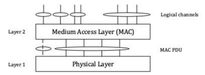
Figure 6.1-1: Radio interface protocol architecture
