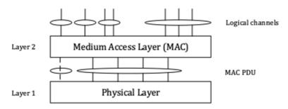
Figure 6.1-1: Radio interface protocol architecture
