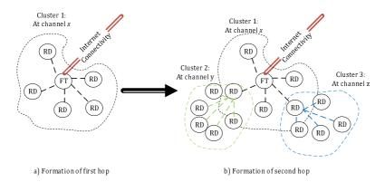
Figure 5.3.2-1: Formation of the clustered tree mesh network topology
