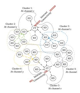
Figure 5.3.2-2: Example formation of the clusters in multiple FT scenario
