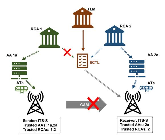
Figure 7: Secured communication when unknow RCA is not included in the ECTL
