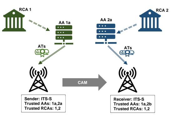
Figure 4: Secured communication using certificates from different PKIs
