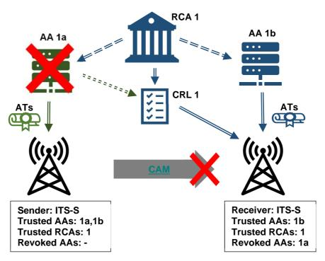
Figure 6: Secured communication using AT issued by AA included in the CRL
