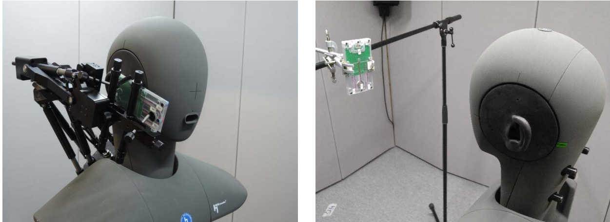
Figure D.3: Test setup for mobile devices: handset (left) and hands-free (right) mode
