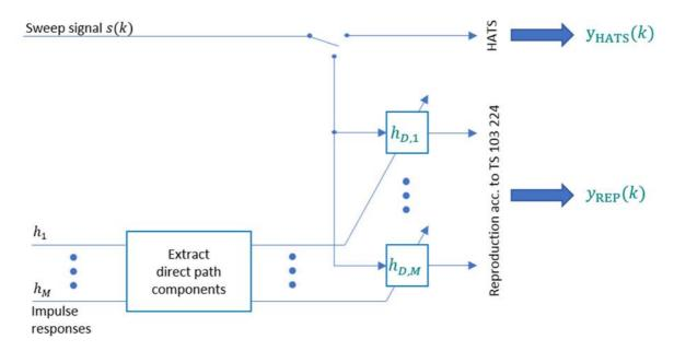
Figure 5: Overview of the signal processing for the delay compensation
