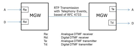
Figure 1: Reference configuration scenario between two MGW
