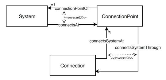
Figure 4: SAREF4SYST: Connection points of systems, where other systems connect
