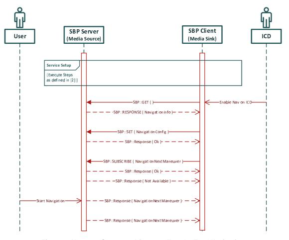
Figure 2: Message Sequence Diagram - Turn-by-Turn Navigation
