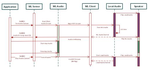
Figure 18: Unblocking of MirrorLink Audio with presence of Local Audio
