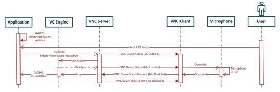
Figure 8: Message Sequence for VC with Occupied Microphone
