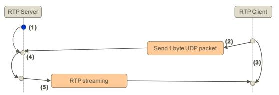
Figure 4: Sequence to Establish the RTP Connection
