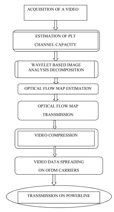
Figure 3: PHDMI general scheme for video compression based on Powerline Channel capacity estimation
