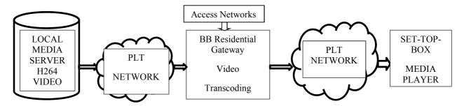
Figure 1: Broadband Residential Gateway with Video Transcoding
