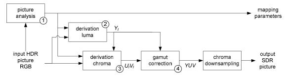
Figure C.1: synoptic of HDR-to-SDR decomposition process.
