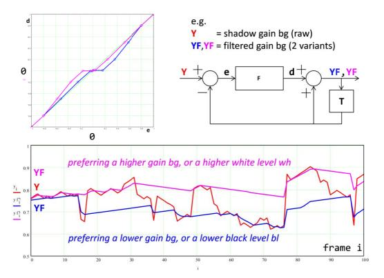
Figure C.10: Example temporal filters for the shadow gain and white level parameters
