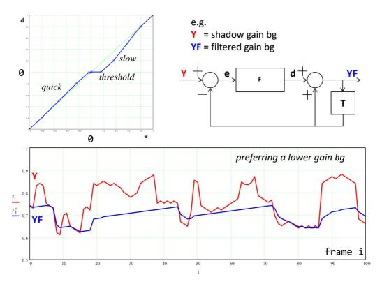
Figure C.9: Example temporal filter for the shadow gain parameter
