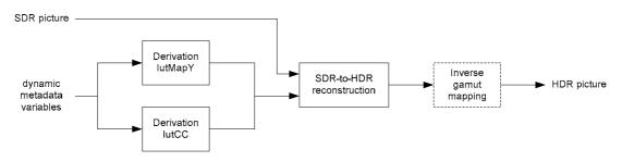
Figure 3: Overview of the HDR reconstruction process.
