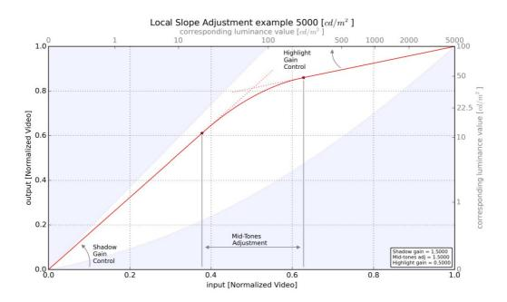
Figure C.5: Tone mapping curve shape example
