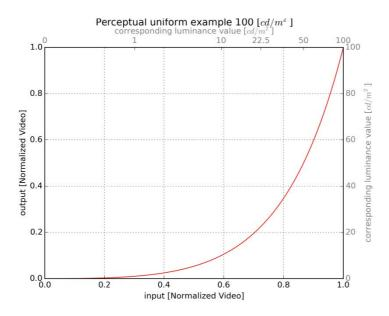
Figure C.7: Perceptual to linear curve based on 100 cd/m<sup>2</sup>
