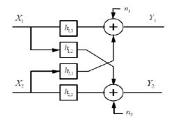
Figure 2: DSL and PLT channel coupling MIMO model
