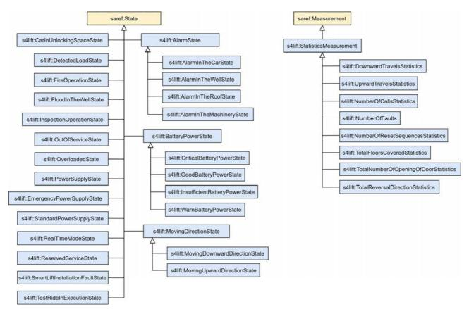
Figure 6.2.4-1: States and measurements model
