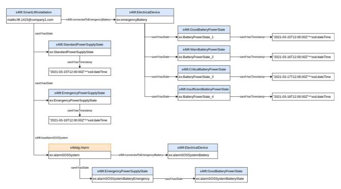
Figure 7-10: Power Supply Signals example
