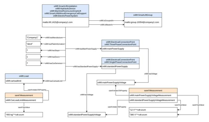
Figure 7-3: Smart Lift Installation example
