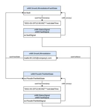
Figure 7-8: Fault Signals example
