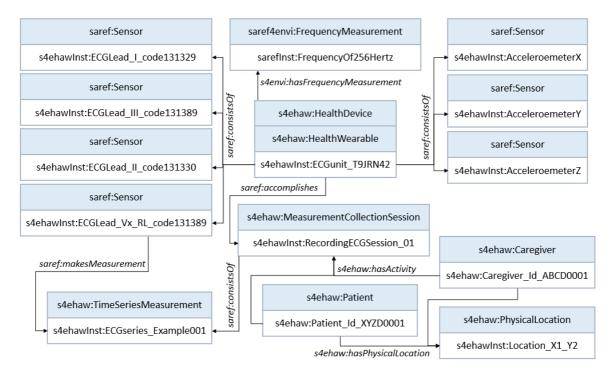
Figure 16: Composition of ECG device with a recording measurement session
