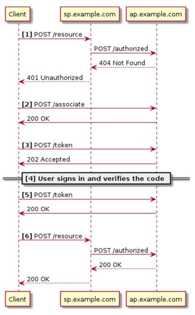
Figure 3: Provision of token for an existing client with a new service provider with pairing code input
