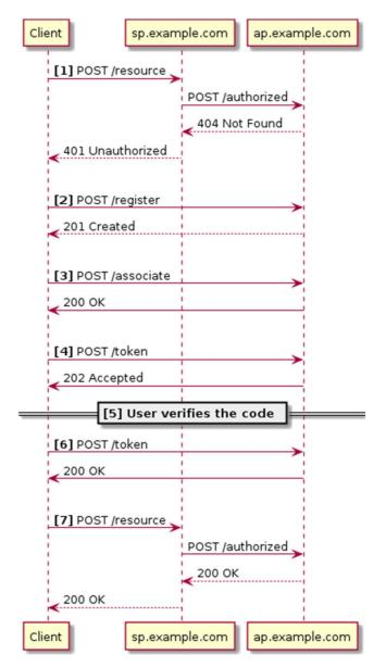
Figure 1: Overview of CPA user mode device flow
