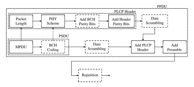
Figure 3: Transmitter Physical Layer Chain
