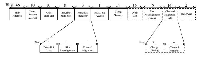
Figure 12: Data Channel Beacon Frame Format
