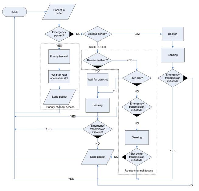
Figure A.1: Flowchart of Multi-use Channel Access
