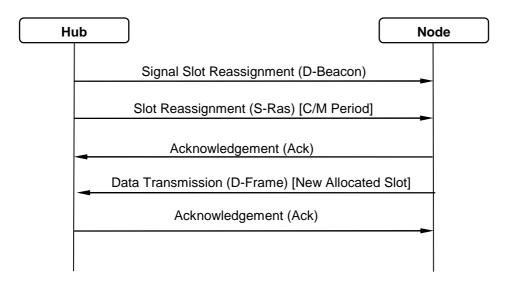
Figure 20: Scheduled Period Slot Reassignment Procedure
