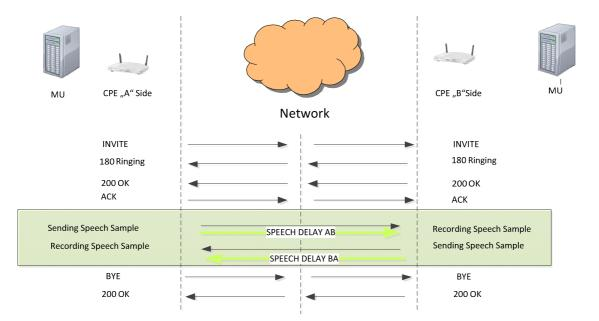
Figure 27: VoIP measurement of the speech delay
