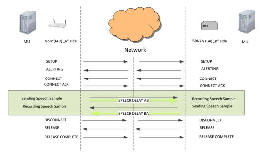
Figure 26: Measurement of the speech delay
