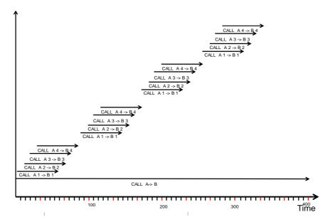
Figure 14: Example of multiple voice channel access test
