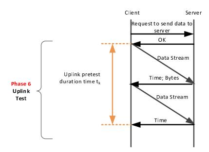
Figure 54: Sample diagram of the Uplink test
