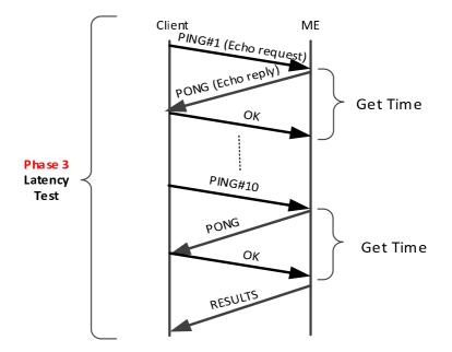
Figure 51: Sample diagram of the Latency test
