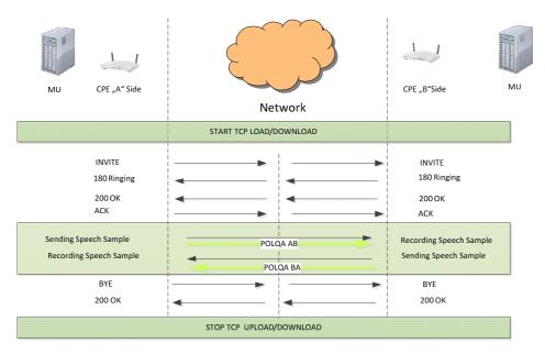
Figure 18: VoIP measurement of voice quality with parallel data load
