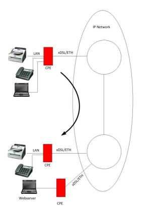
Figure 37: Call between two MMTel (IMS) Fax UE with additional data traffic
