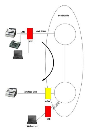
Figure 38: Call between MMTel (IMS) Fax UE with additional data traffic and AGW Fax UE
