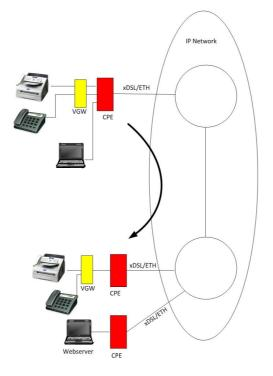
Figure 40: Call between two VGW Fax UE with additional data traffic
