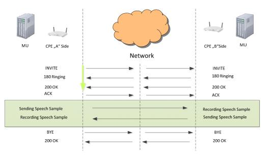
Figure 9: VoIP: determination of the call drop ratio
