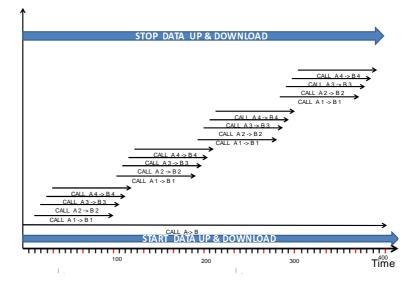
Figure 23: Multiple voice channel access test
