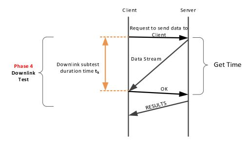
Figure 52: Sample diagram of Downlink tests depicting one TCP stream
