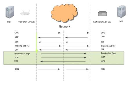
Figure 29: Fax setup duration
