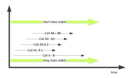
Figure 24: Parallel quality measurement of multiple voice channels and data transmission speed
