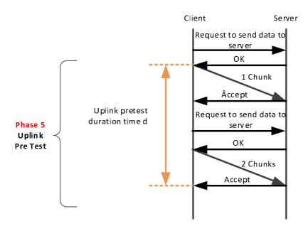
Figure 53: Sample diagram of the Uplink pre-test
