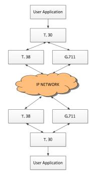
Figure 28: FAX Stack for FoIP
