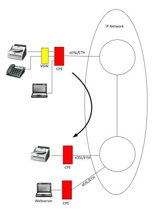
Figure 42: Call between VGW Fax UE with additional data traffic and MMTel (IMS)
