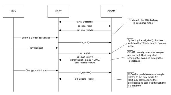
Figure 7: Playback execution sequence diagram
