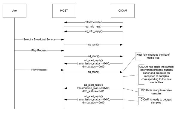
Figure 8: Playback re-start sequence diagram
