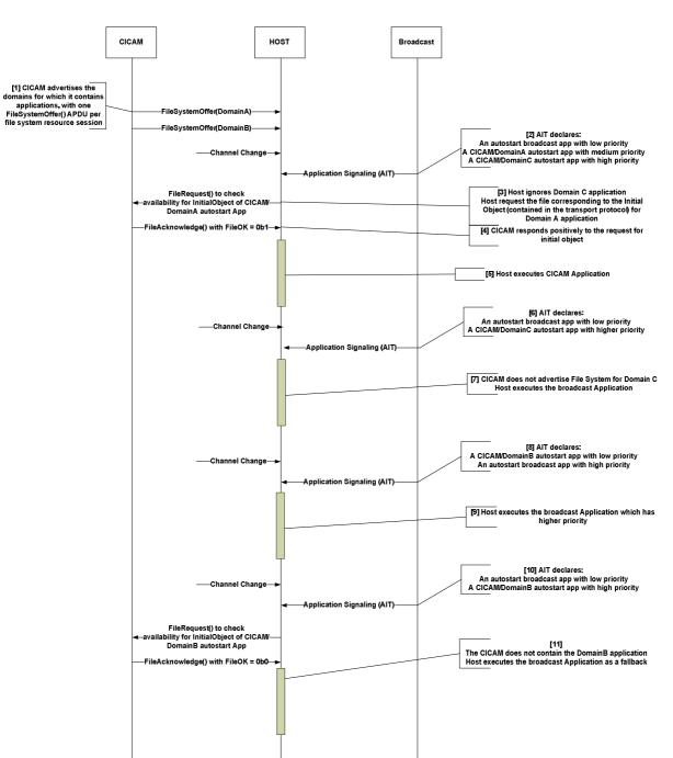
Figure 22: Broadcast signalled application launch example
