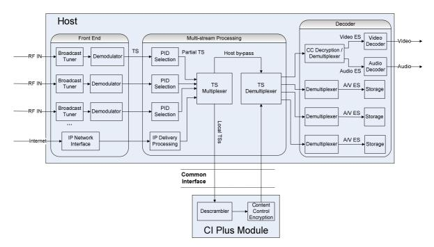
Figure 3: CI Plus extended architecture for multi-stream reception
