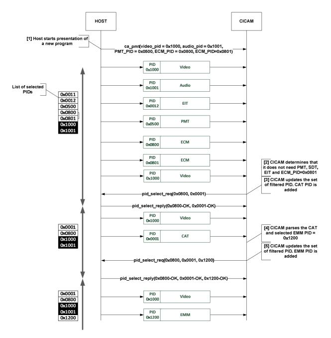
Figure 4: PID selection example sequence diagram
