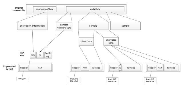
Figure 17: Encapsulation of ISOBMFF content into a TS
