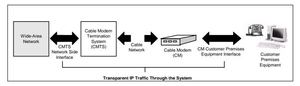
Figure 1: Transparent IP Traffic Through the Data-Over-Cable System
