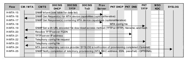
Figure 9: Embedded-MTA Hybrid Power-on Initialization Flow
