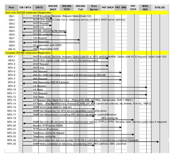
Figure 6: Embedded-MTA Secure Power-on Initialization Flow (IPv4 eCM)
