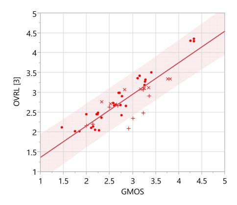
Figure 36: G-MOS fit to OVRL BAK after 3<sup>rd</sup> order mapping, English results, shaded area is 95 % confidence interval
