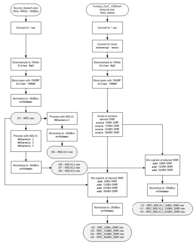
Figure D.2: Wideband processing for reference set
