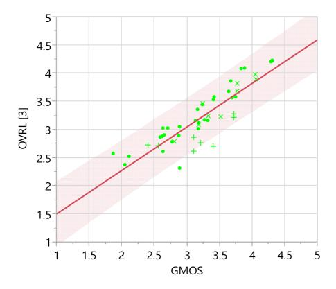
Figure 34: G-MOS fit to OVRL BAK after 3<sup>rd</sup> order mapping, Chinese results, shaded area is 95 % confidence interval
