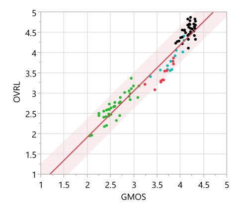
Figure 53: G-MOS fit to OVRL, Tests 5 and 6, shaded area is 95 % confidence interval
