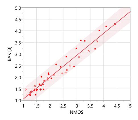
Figure 32: N-MOS fit to BAK after  $3^{\rm rd}$  order mapping, English results, shaded area is 95 % confidence interval
