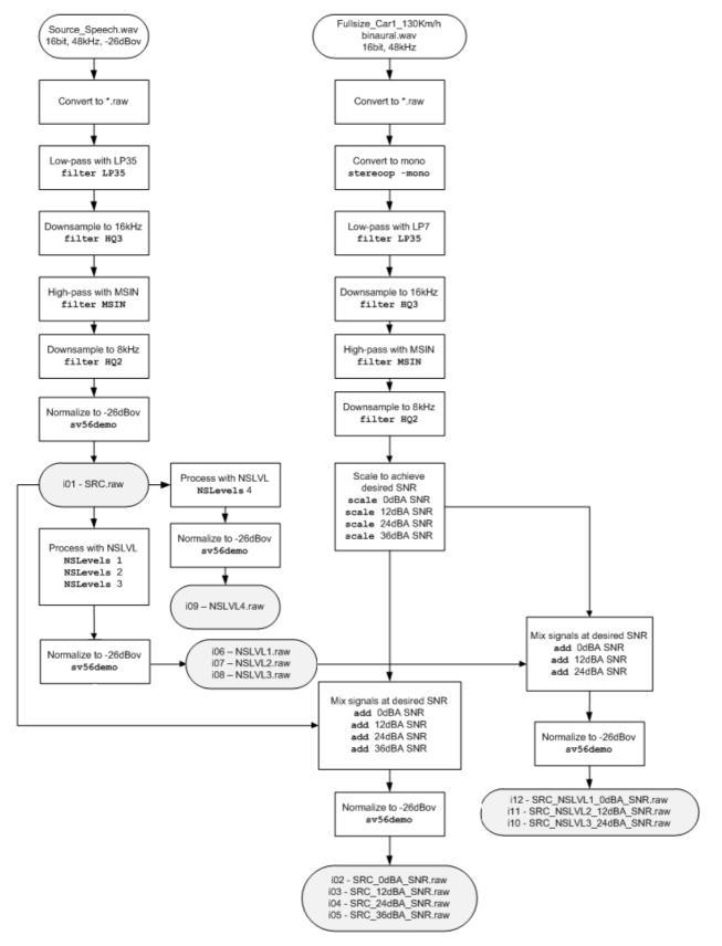
Figure D.3: Narrowband processing for reference set
