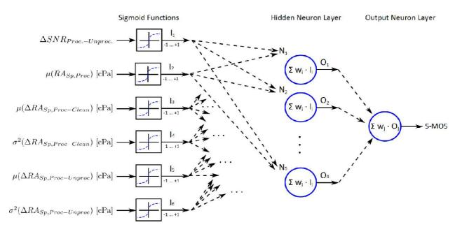
Figure 1: Structure of neural network for S-MOS
