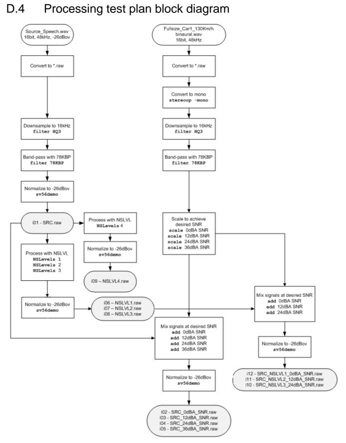
Figure D.2: Wideband processing for reference set
