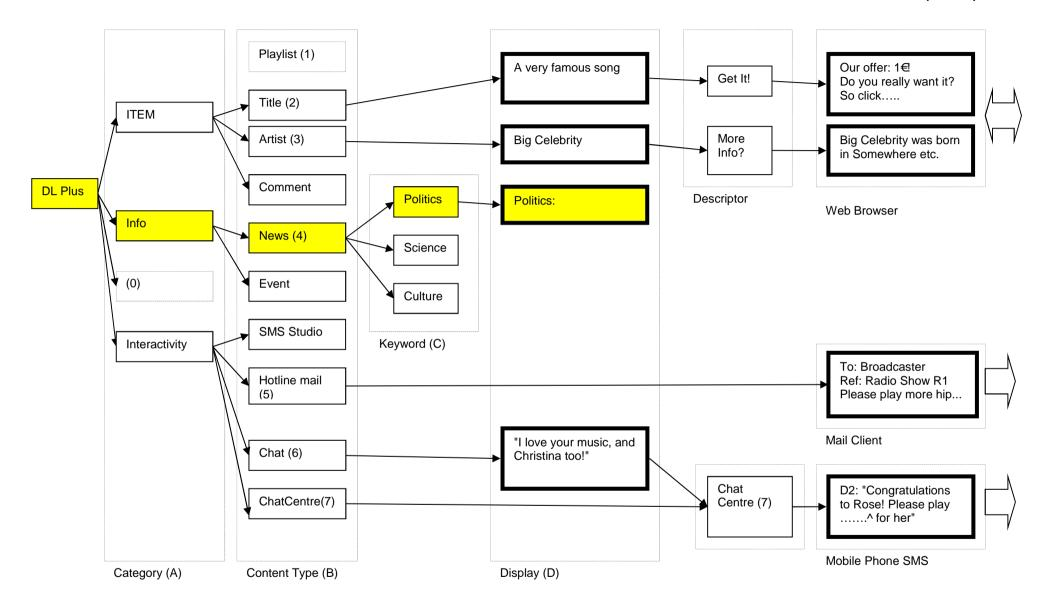
Figure B.1: Navigation through DL Plus objects stored in a receiver; Display of DL Plus objects; Display of linked applications: Web Browser, Mail Client, SMS Client
