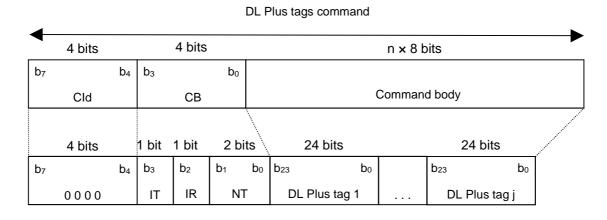
Figure 8: Structure of the DL Plus tags command
