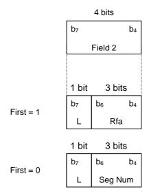
Figure 6: Structure of Field 2 for DL Plus
