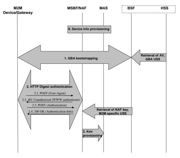
Figure 6.1: M2M Service Bootstrap based on GBA
