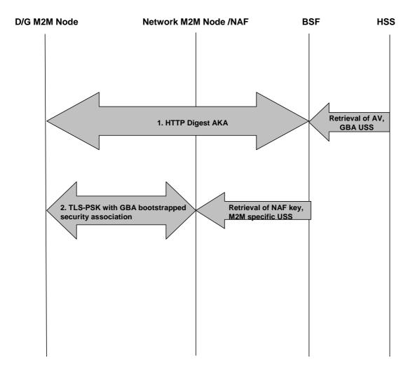
Figure 7.1: M2M Service Connection based on GBA
