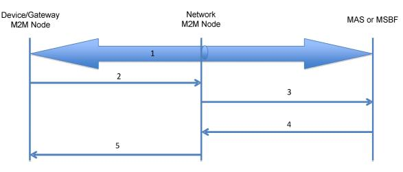
Figure 6.5: D/G M2M Node-initiated M2M Bootstrap-Erase Procedure
