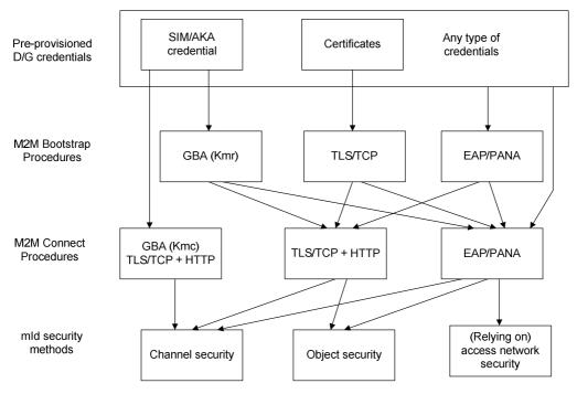
Figure I.1: Security credential and method combinations
