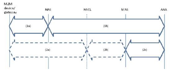
Figure 6.2: Bootstrapping via network access authentication
