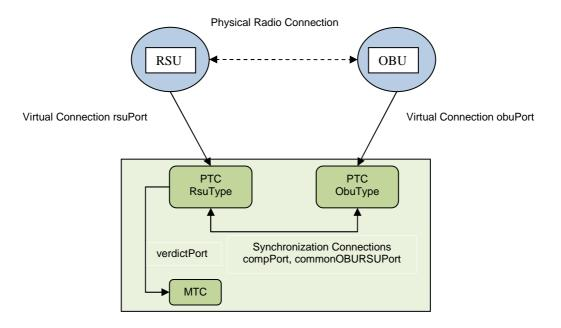
Figure 1: Test architecture
