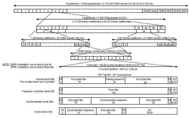
Figure 10: Overall Burst structure of a GSM System
