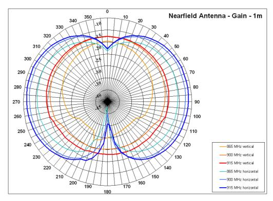
Figure 7: Measured antenna diagram of an antenna used in PoS and packaging applications
