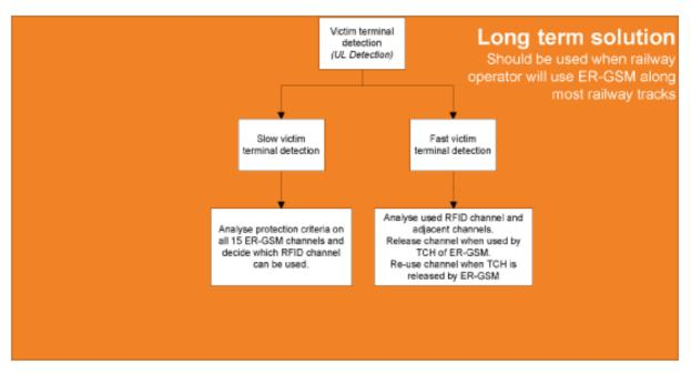
Figure 17: Additional mechanisms for the long term solution for the sharing in the band 918 MHz and 921 MHz
