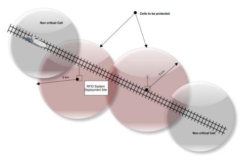
Figure 16: ER-GSM network coverage
