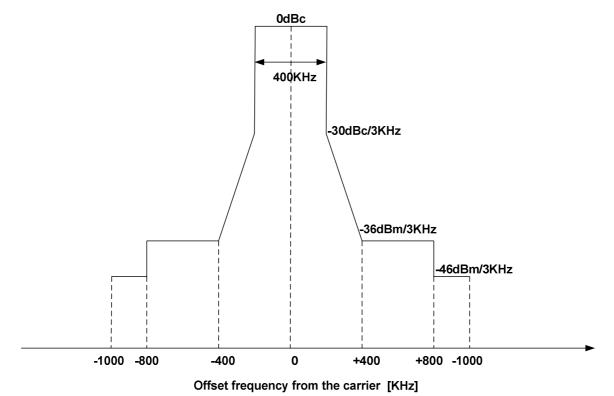
Figure C.2: High performance interrogator channel mask
