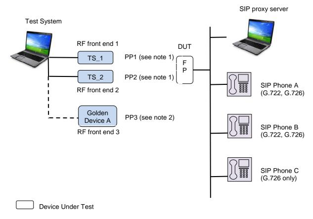
NOTE 1: PP1 and PP2 behave either as a NG PP, a legacy GAP PP, or a headset PP according to test case.
