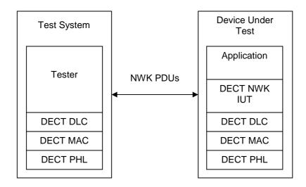
Figure 1: New Generation DECT remote test method
