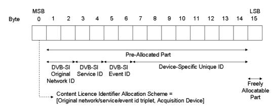
Figure 6: CLID allocation scheme for DVB broadcast event and Acquisition Device
