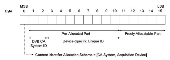
Figure 8: CLID allocation scheme for CA system and Acquisition Device
