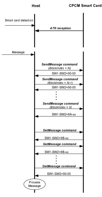
Figure 5: CPCM Commands exchange example
