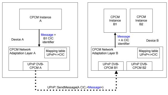
Figure 1: typical behaviour of the DVB-HN NAL for CPCM
