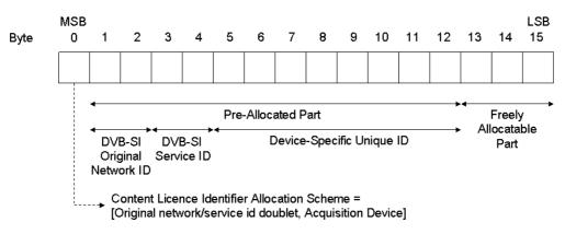
Figure 7: CLID allocation scheme for DVB broadcast service and Acquisition Device
