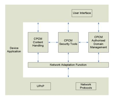
Figure 2: ADM Interfaces to other CPCM Sub-systems
