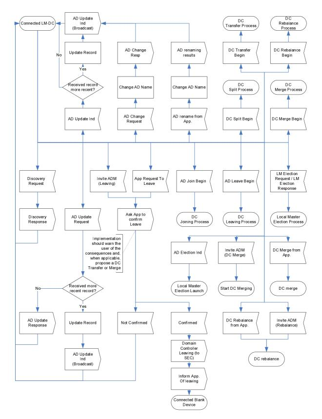
Figure 11: Connected Local Master and Domain Controller State Machine
