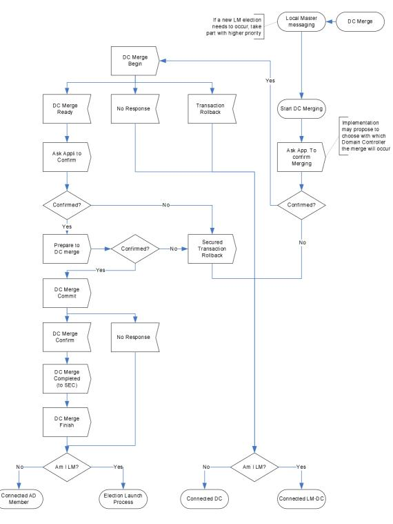
Figure 25: Merging Domain Controller
