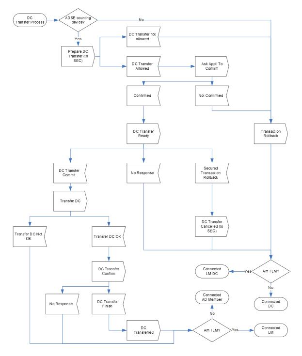
Figure 22: Domain Controller transfer
