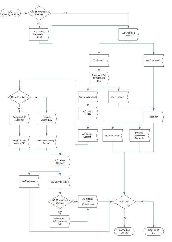
Figure 20: Domain Controller in AD Leaving Process
