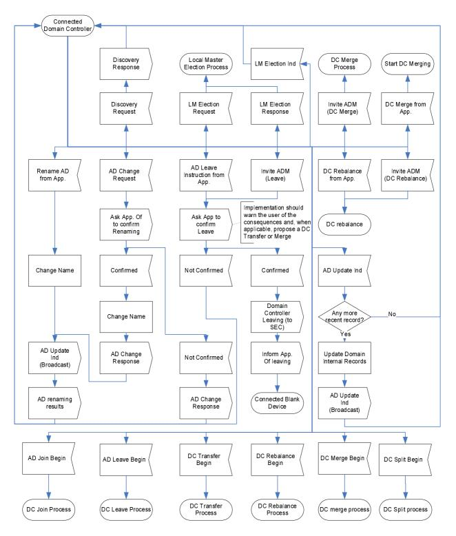
Figure 9: Connected Domain Controller State Machine
