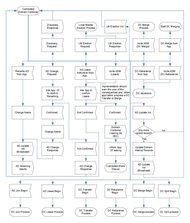
Figure 9: Connected Domain Controller State Machine
