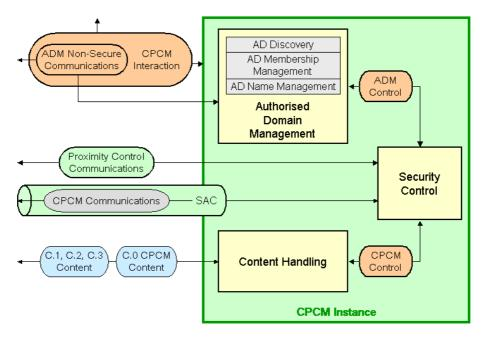
Figure 1: ADM in the CPCM Reference Model
