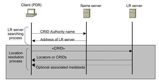
Figure 12.3: Example of location resolution server discovery
