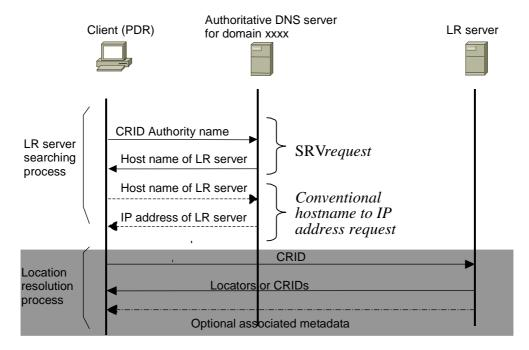
Figure 12.4: Stages of TCP/IP based resolution server discovery
