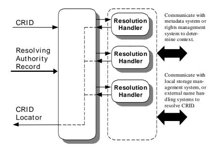
Figure 12.1: CRID resolution architecture
