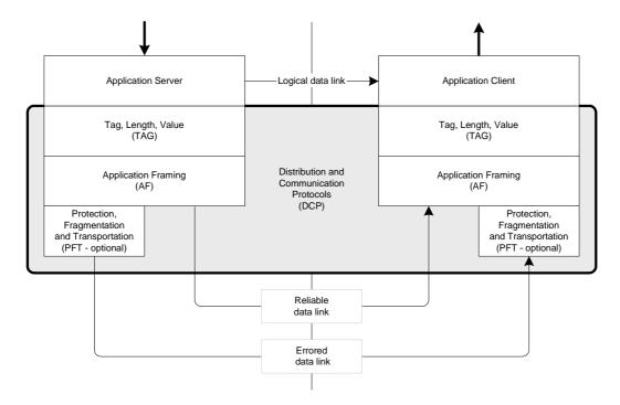
Figure 1: DCP protocol stack
