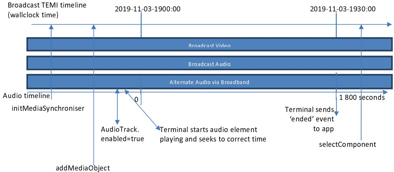
**Figure M.2: Example of alternate audio track for a broadcast TV service**
