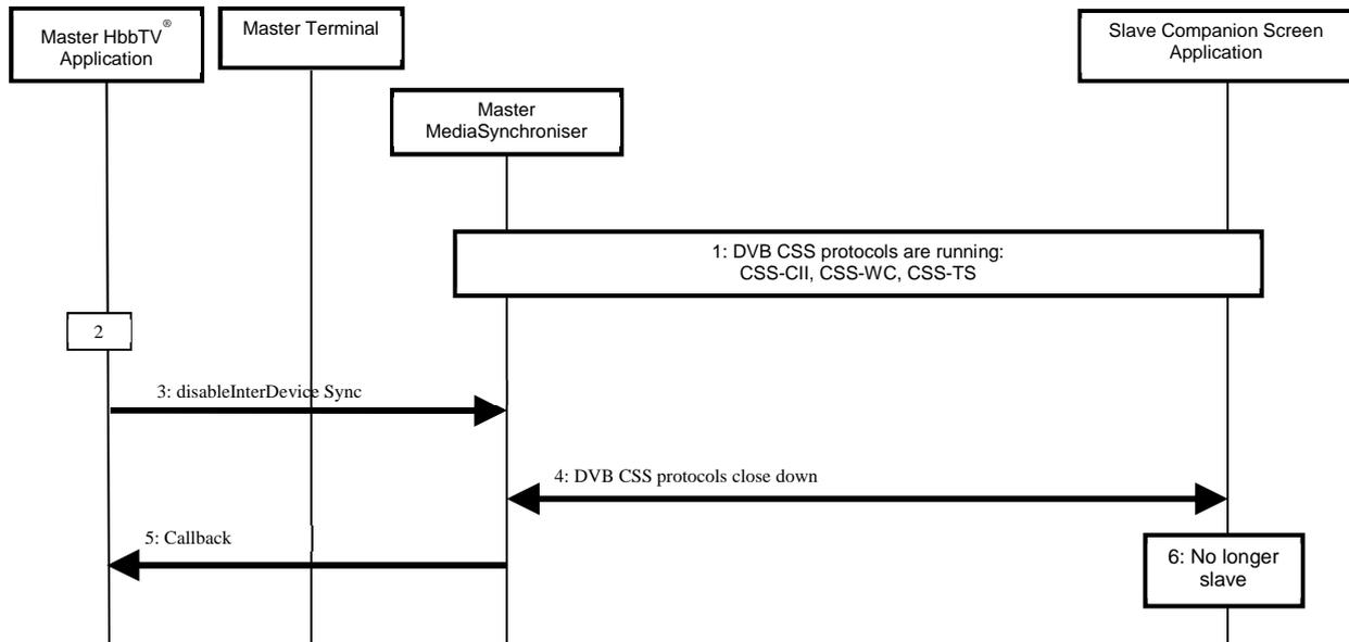
**Figure 29: Termination of inter-device timeline synchronization**
