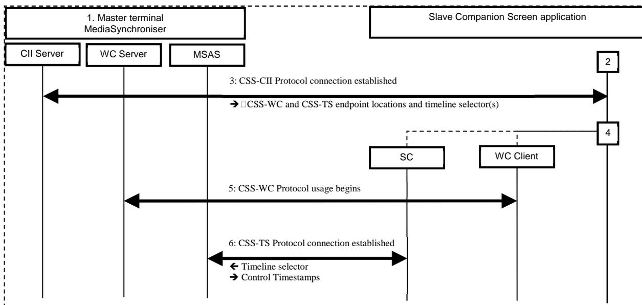
**Figure 28: Protocol interactions for inter-device timeline synchronization**
