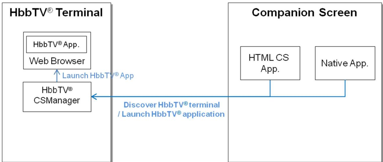
**Figure 36: Architecture for remotely launching HbbTV<sup>®</sup> applications**
