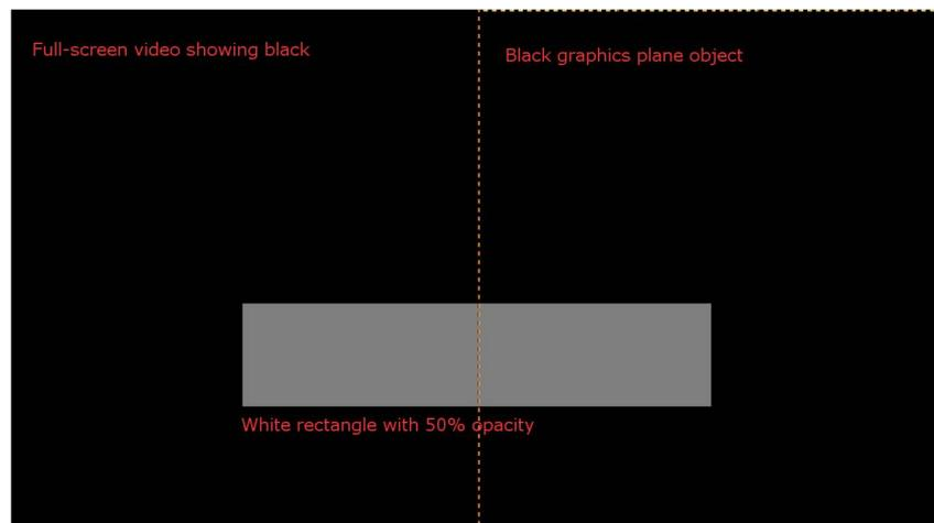
Figure 17: Example for a correct rendering of video and graphics
