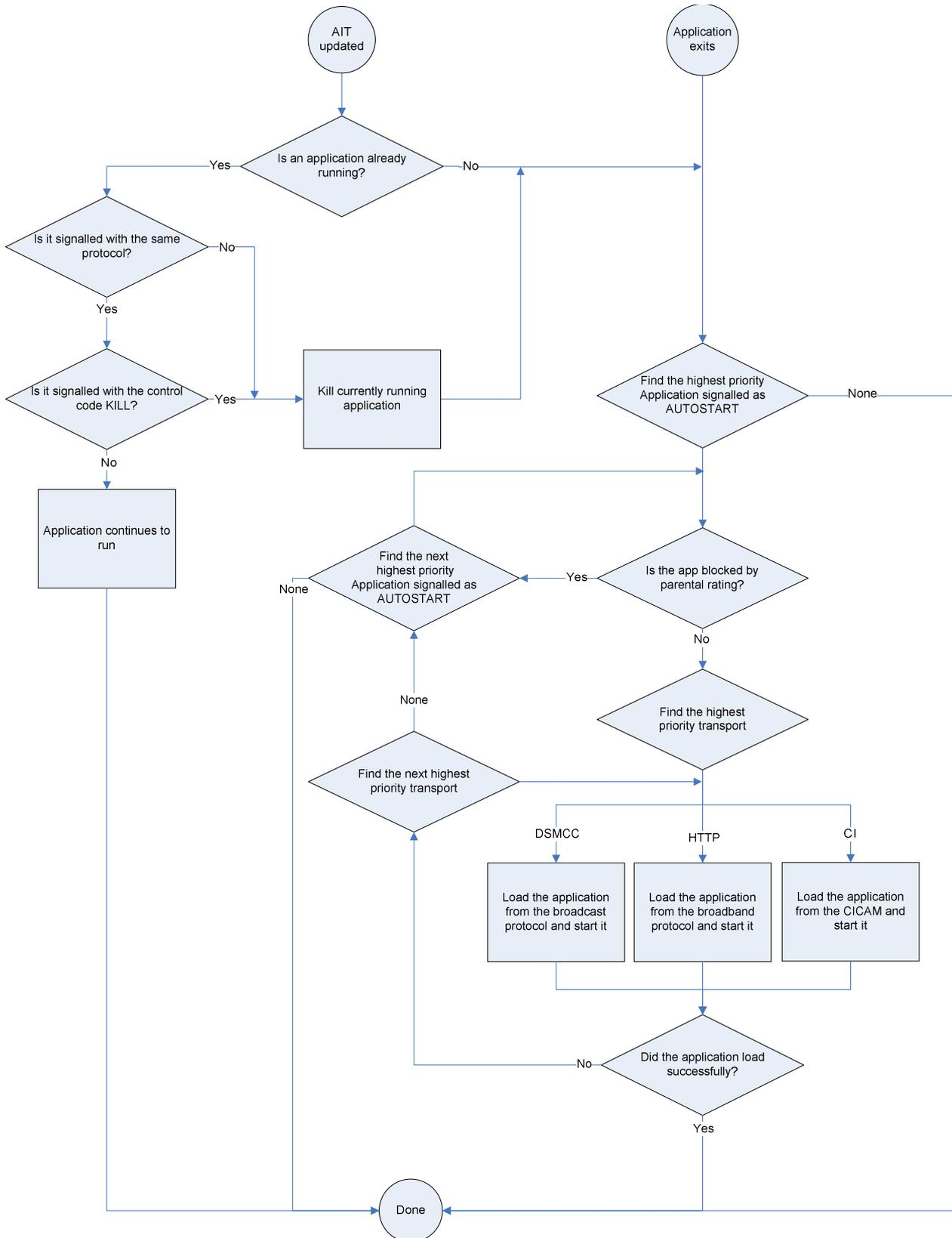
Figure 14: Behaviour while a broadcast service is selected
