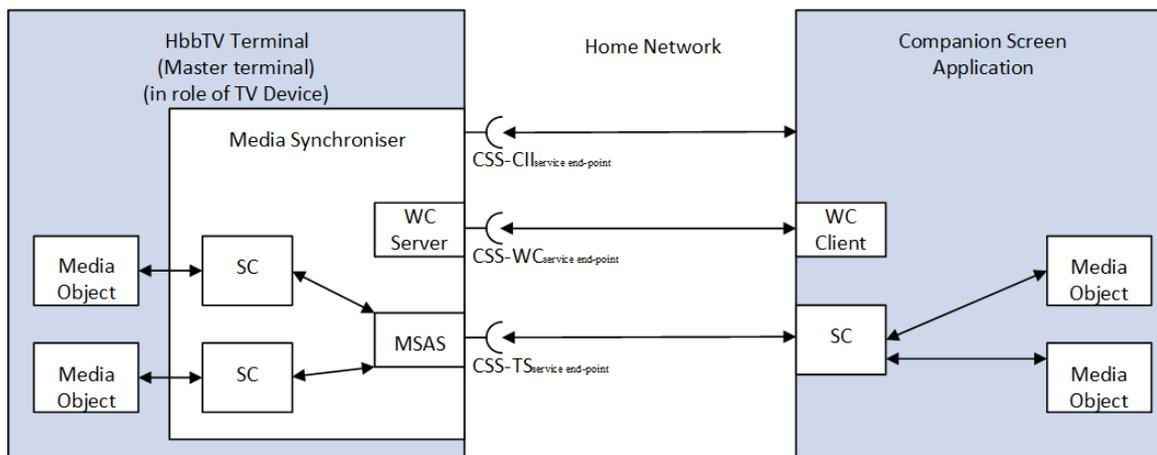
**Figure 25: Relationship between the HbbTV<sup>®</sup> MediaSynchroniser and MSAS, SC, WC Server and WC Client elementary functions and protocol service endpoints**
