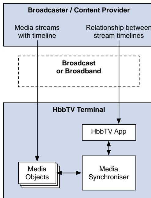
**Figure 20: Relationship between `MediaSynchroniser` object and HbbTV<sup>®</sup> application for multi-stream synchronization**
