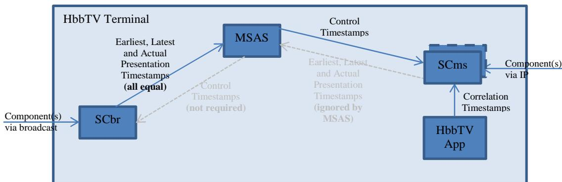
**Figure G.4: Multi-stream Media Synchronization with no buffer for broadcast within the HbbTV<sup>®</sup> terminal**
