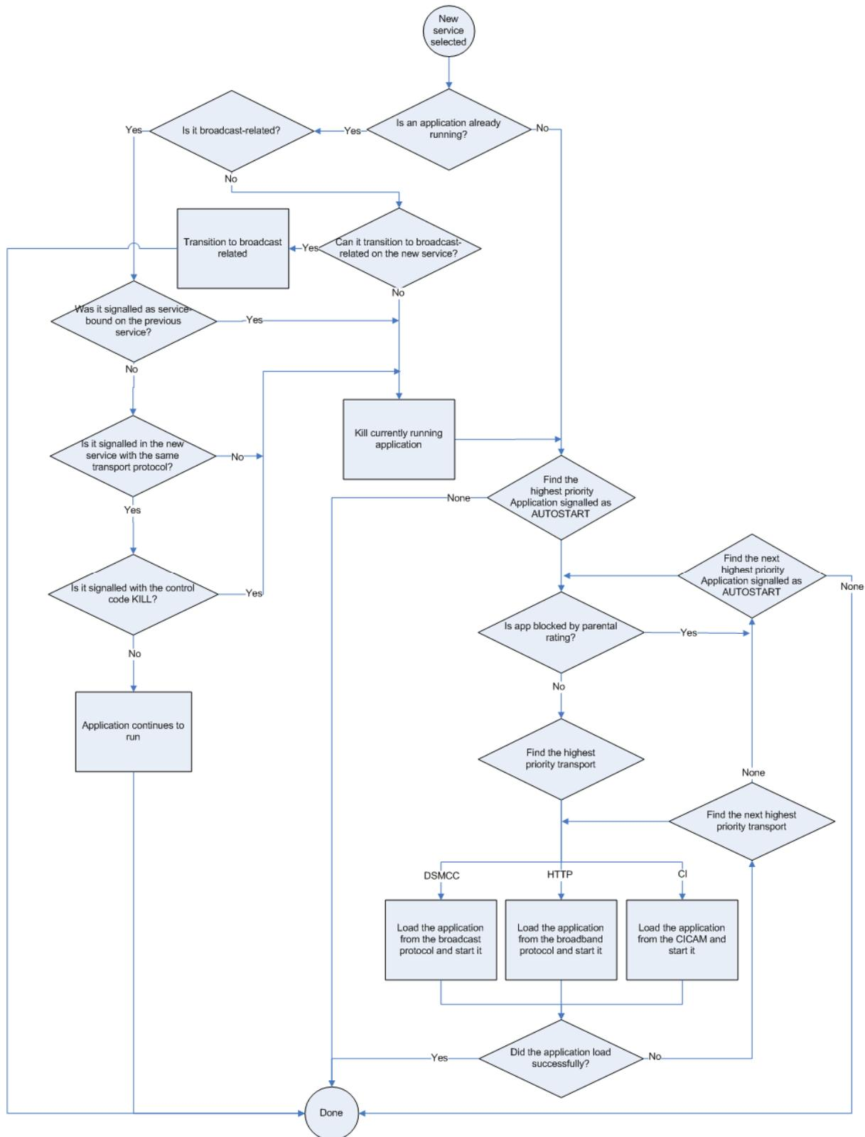
Figure 13: Behaviour when selecting a broadcast service
