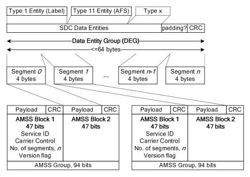
Figure A.1: The AMSS block and Data Entity Group structure
