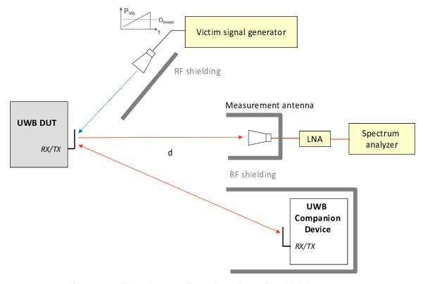
Figure G.1: Exemplary configuration of a radiated DAA test setup
