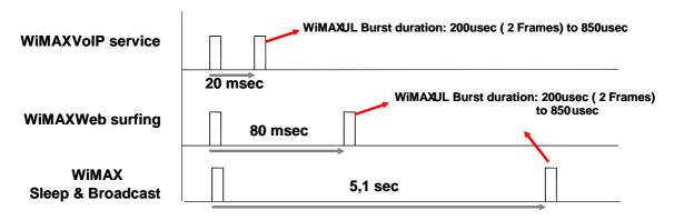
Figure 7: Typical BWA timing patterns for victim signal emulation
