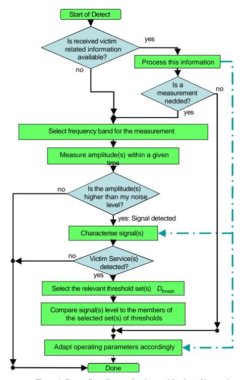
Figure 6: Detect flow diagram for the combination of internal measurements and external information
