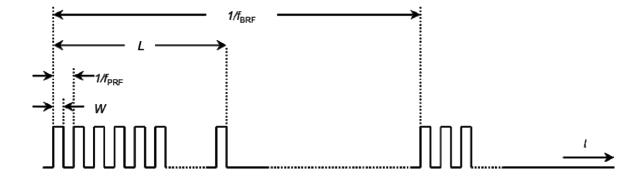
Figure D.5: General structure of the bursts for DAA radiolocation test transmissions
