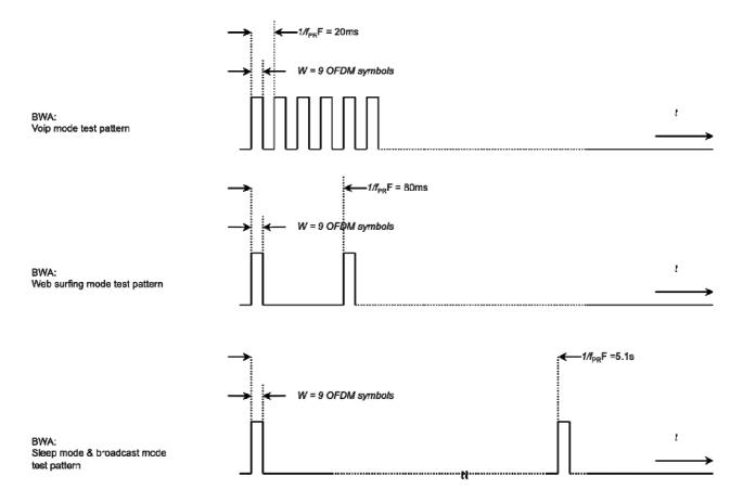
Figure E.1: Timing of BWA test signals
