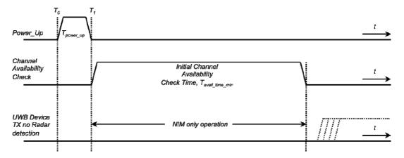
Figure D.1: Example of timing for radiolocation testing of the Minimum Initial Channel Availability Check Time  $T_{\text{avail time}}$ , UWB DAA devise intent to operate in a non NIM mode
