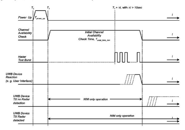
Figure D.3: Example of timing for radar testing towards the end of the Minimum initial Channel Availability Check Time
