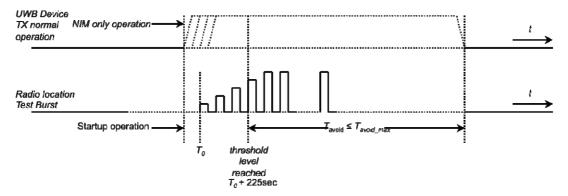
Figure D.4: Example of timing for radiolocation signal in-operation testing of the Detect and Avoid Time, here with increasing Radiolocation test signal level larger than the threshold
