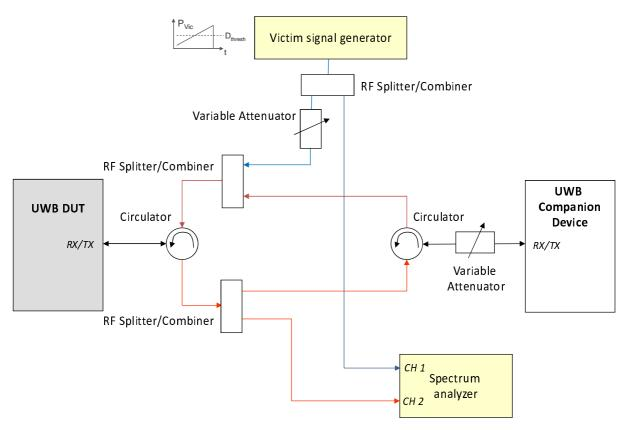
Figure G.2: Exemplary configuration of a conducted DAA test setup
