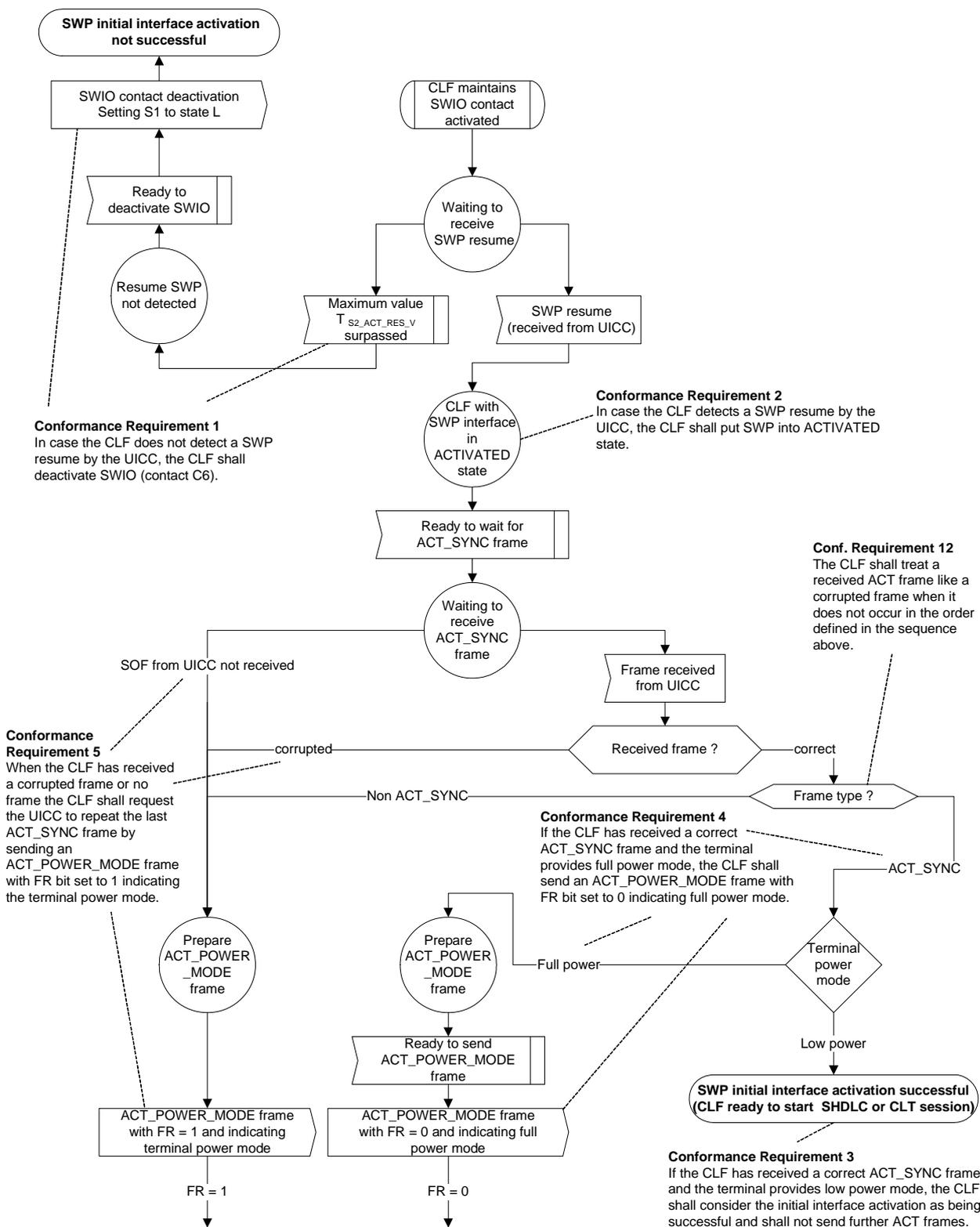
Figure A.2.1: Initial SWP interface activation, part 1
