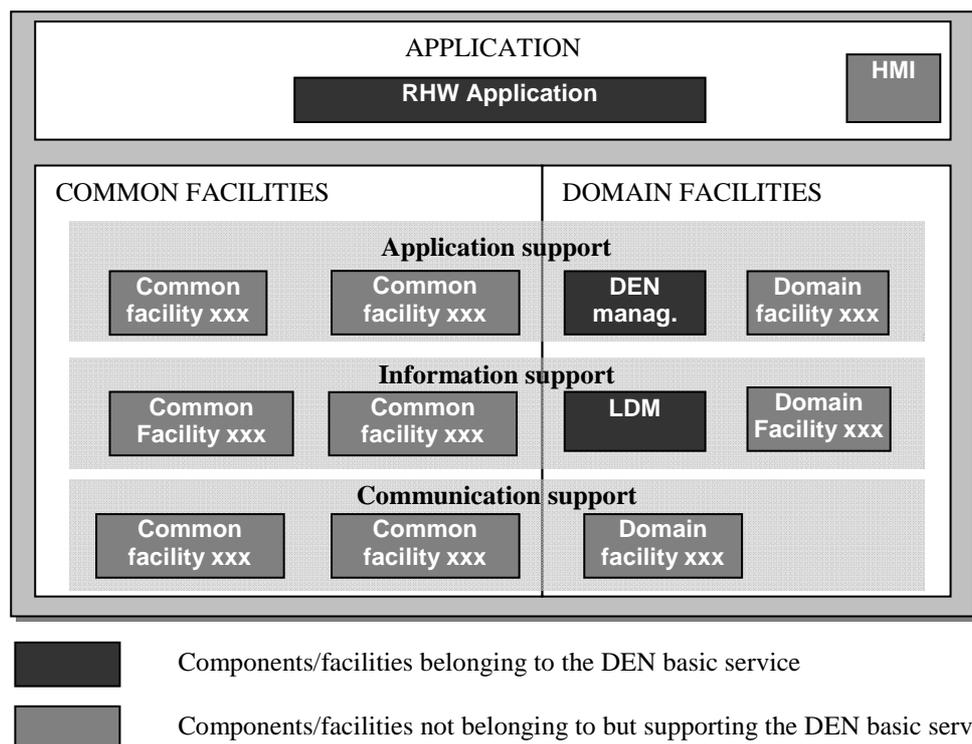
**Figure 1: DEN basic service components**
