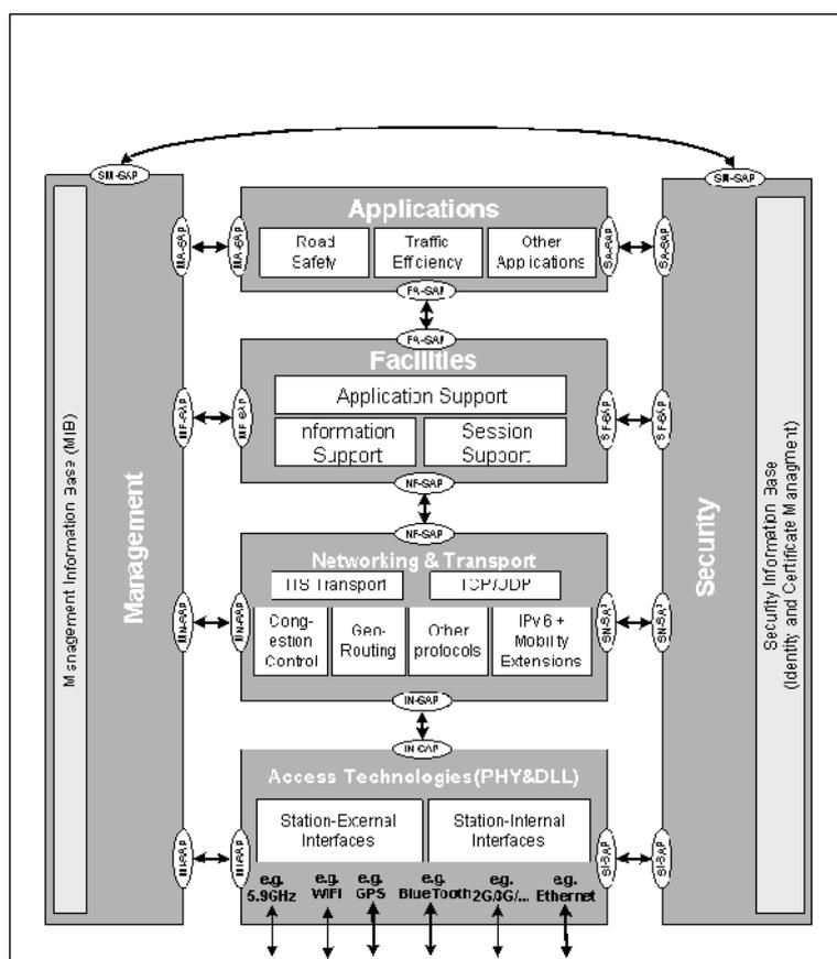
Figure 1: ITS Station Reference Architecture
