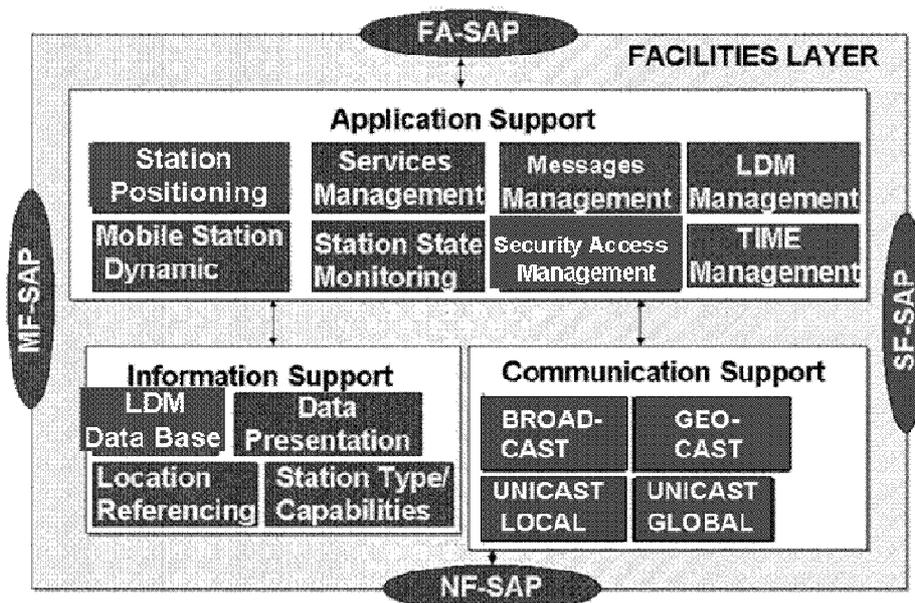
Figure 2: Facilities Layer Architecture
