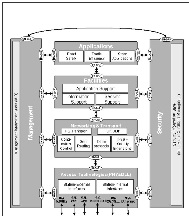
Figure 1: ITS Station Reference Architecture
