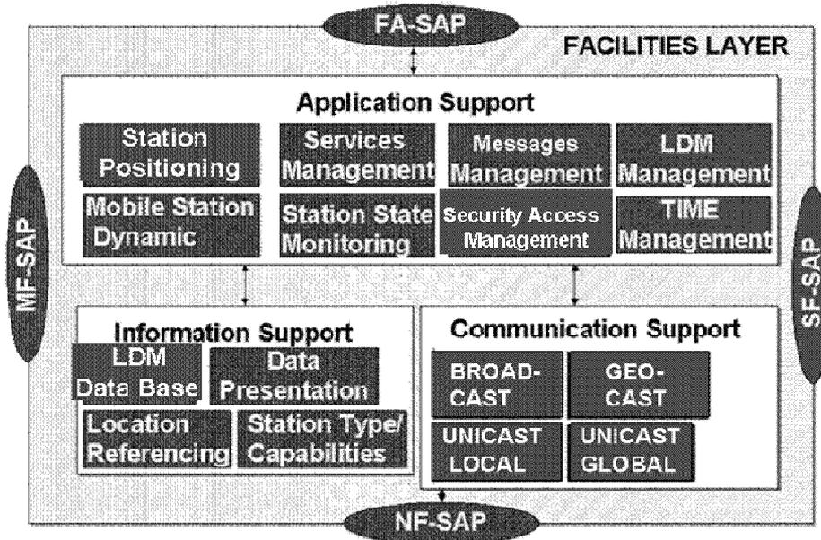
Figure 2: Facilities Layer Architecture
